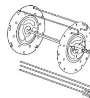
To extract when cooking finished, keep the unlock button (15) to the right and with the handle (12) lift up the accessory and extract it.
