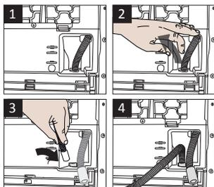
**i** Water drain hose should be attached to a height of maximum 80 cm.
