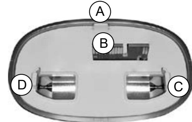
Pay attention to the direction of insertion. There are 3 plastic pivot hinges (A C D) found behind the light and an electronic card (B). During installation of the light, be careful to match these elements with their corresponding housings on the machine's attachment. Installation and removal of the light does not require equipment and is hand-made when the Machine is off and disconnected from the power socket.
