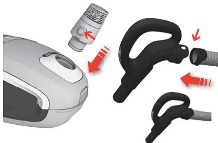
2. **Insert the hose** (to remove it, press the lock buttons and pull the hose out). Insert the hose into the hose handle until the catches click to engage (press the catches to release the hose).
