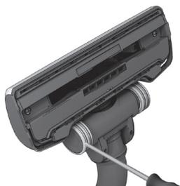
2. **If the wheels are stuck**, clean them by removing the wheel cap with a small screwdriver.
