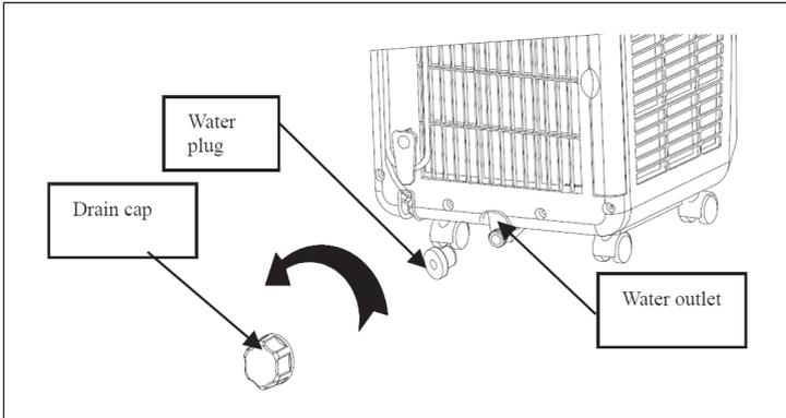
**Note:** Protect the drain cap and water plug properly. Tilt the unit slightly backward when draining. Turn on the unit only after the water plug and drain cap are installed properly; otherwise, the condensate of the unit will flow onto the ground or carpet.
