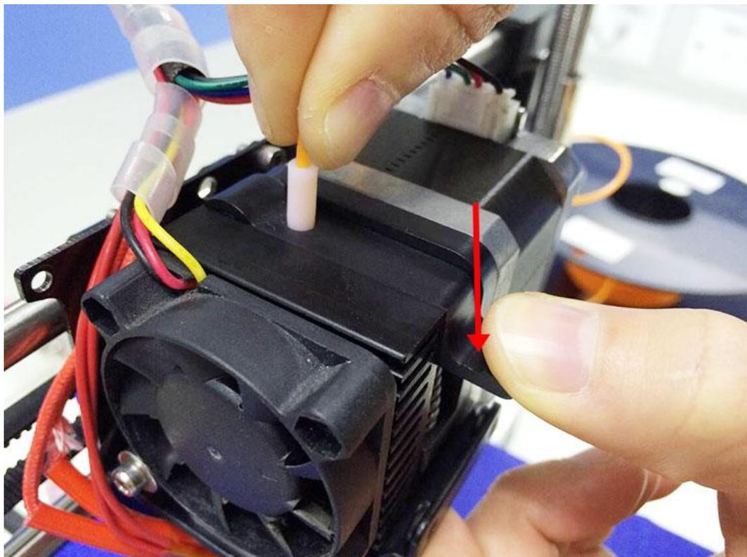
After pushing the filament into the bottom of hotend, use the feeding button on Repetier (as shown
