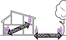
The operating range is up to 50 meters / 165 feet indoors and 300 meters / 985 feet outdoors. The operating range of the baby monitor varies depending on the surroundings and factors that cause interference. Wet and moist materials cause so much interference that the range loss is up to 100%.
