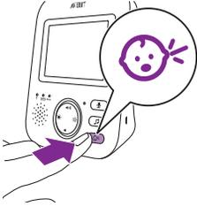
The sensitivity level of the baby unit defines what you hear through the parent unit. When the level is set high, you will hear many sounds, including soft background sounds. When the sensitivity level is set low, you will hear only the louder sounds.
