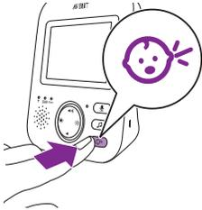
1 Press the sensitivity button to access the sensitivity levels.
