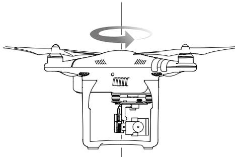
3. Hold the aircraft with its camera facing down, and rotate it 360 degrees along its central axis. The Aircraft Status Indicator will change from solid green to flashing yellow when complete. The calibration is successful.
