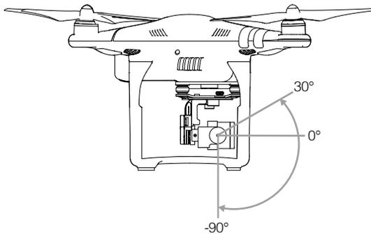
Use the gimbal dial on the remote controller to control the tilt motion of the camera.
