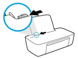
3. Insert one or more envelopes into the far-right side of the input tray and slide the stack of envelopes down until it stops.
