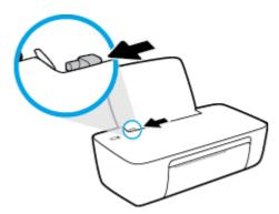
3. Insert a stack of paper into the input tray with the short edge down and the print side up, and slide the stack of paper down until it stops.
