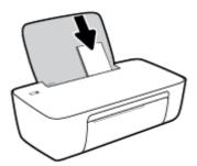
4. Slide the paper-width guide to the right against the stack of envelopes until it stops.
