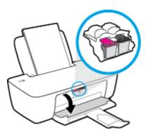
**b.** Press down to release the ink cartridge, and then remove it from the slot.
