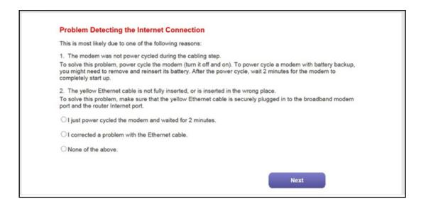
**Note:** The option for power cycling the modem router that is stated onscreen applies to a DSL Internet connection only (see *Set Up Your Modem Router for DSL Service* on page 21).
