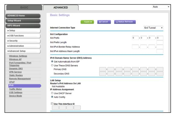
The modem router automatically detects the information in the **Router's IPv6 Address on LAN** field. This field shows the IPv6 address that is acquired for the modem router's LAN interface. The number after the slash (/) is the length of the prefix, which is also indicated by the underline (\_) under the IPv6 address. If no address is acquired, the field displays Not Available.
