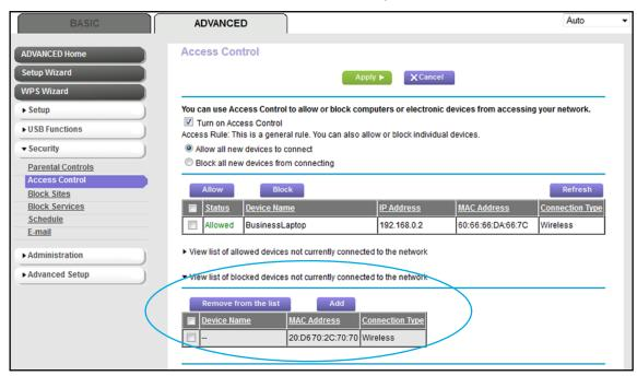
A table displays the detected device names, MAC addresses, and connection types of the devices that are not connected and blocked from accessing the network.
