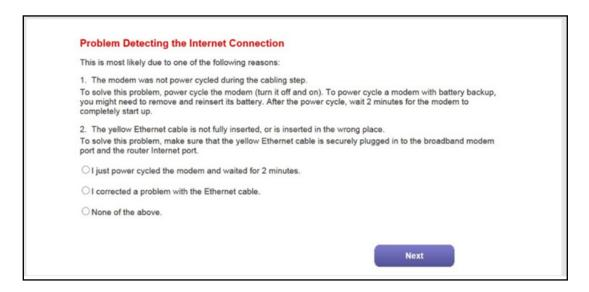
**Note:** The option for the Ethernet cable connection that is stated onscreen applies to a cable or fiber Internet connection only (see *Set Up Your Modem Router for Cable or Fiber Service* on page 29).
