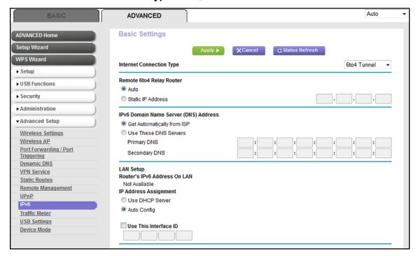
The modem router automatically detects the information in the Router's IPv6 Address On LAN field. This field shows the IPv6 address that is acquired for the modem router's LAN interface. The number after the slash (/) is the length of the prefix, which is also indicated by the underline ( ) under the IPv6 address.
