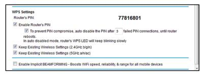
The **Router's PIN** field displays the fixed PIN that you use to configure the modem router's WiFi settings from another platform through WPS.
