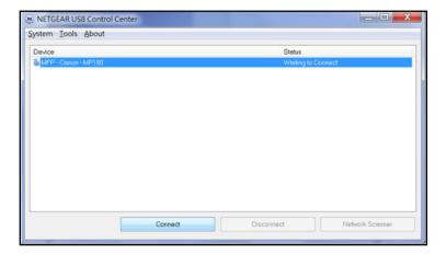
Some firewall software, such as Comodo, blocks NETGEAR USB Control Center from accessing the USB printer. If you do not see the USB printer displayed on the page, you can disable the firewall temporarily to allow the utility to work.
