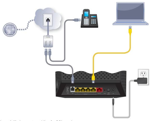
Figure 6. Modem router cabling for DSL service
