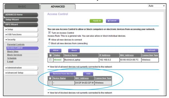
A table displays the detected device names, MAC addresses, and connection types of the devices that are not connected but allowed to access the network.
