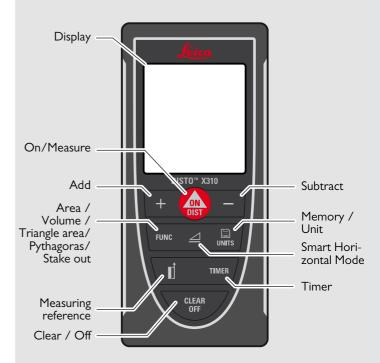
Instrument Set-up EN
